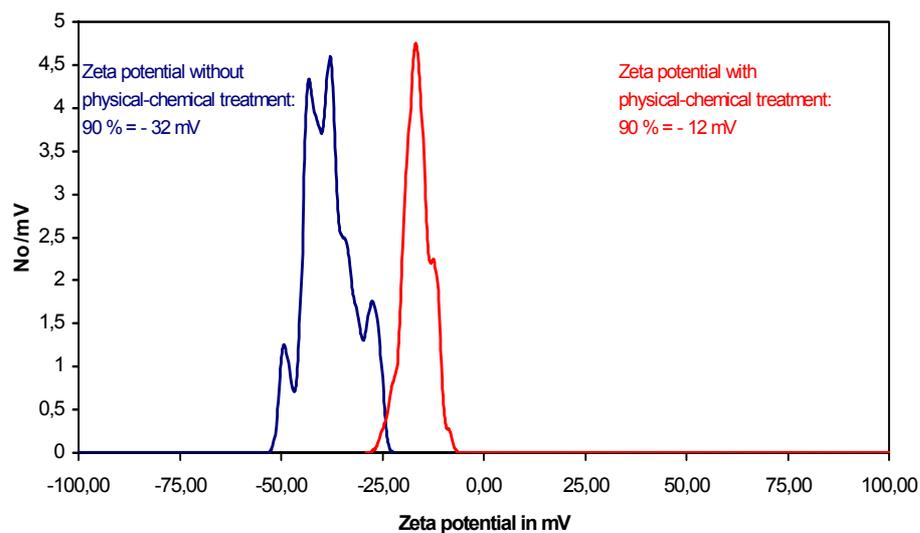
Figure 4: Zeta potential of activated sludge with and without physical-chemical treatment
