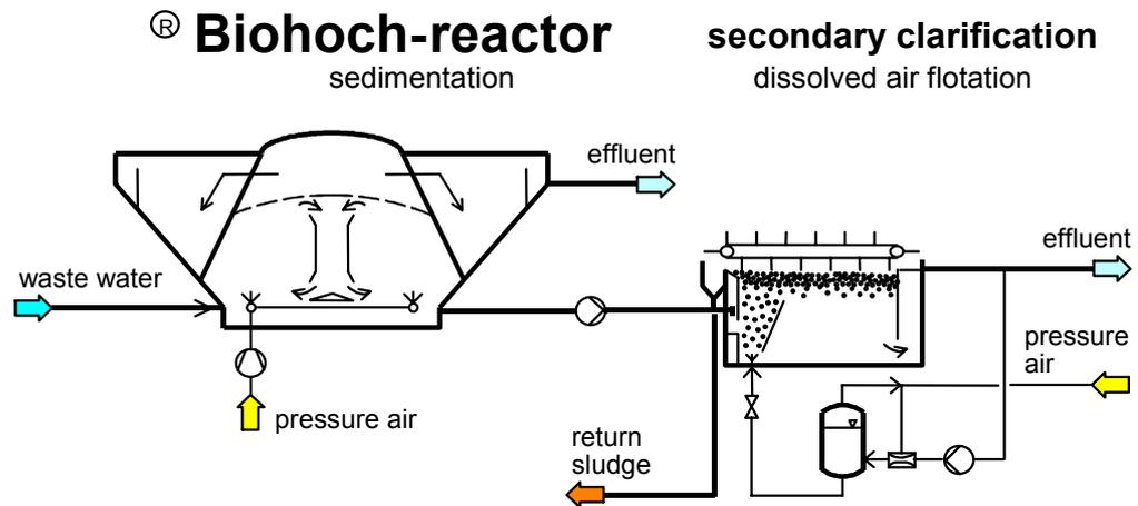
Figure 3: Industrial waste water treatment plant
