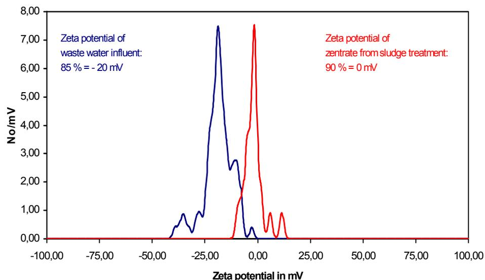
Figure 6: Zeta potential of solids and activated sludge in waste water and centrate from sludge treatment
